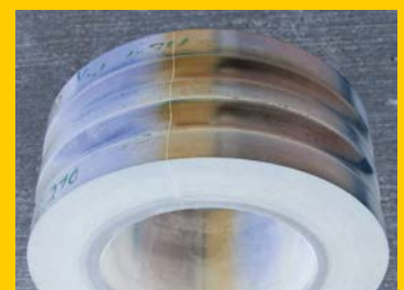
Defective roller with crack
